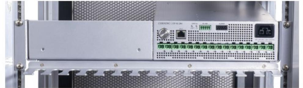
16 Port CIP in 1.5U Tray with Blank Panel and 0.5 RU Routing Guide
